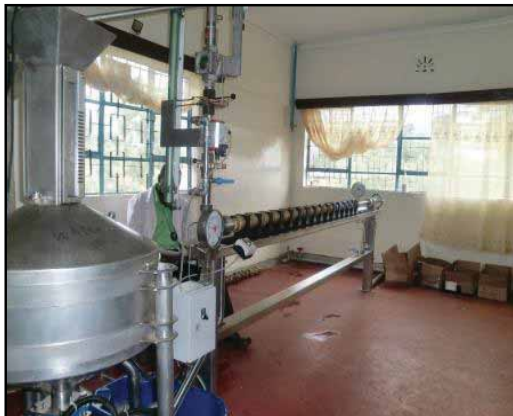
Water Meter Test Bench (NYEWASCO)
